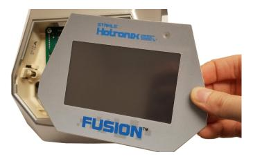
Remove the face board and set safely to the side.
