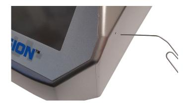
Insert the Paper Clip into the small hole on either side of the housing.
