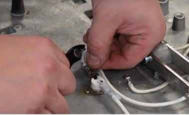
Remove the shrink wrap from the thermostat disc if present.
