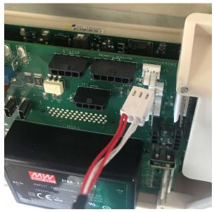
Disconnect the 2-pin Proximity Sensor from the top 2 wire pins using the depressing locking clip.
