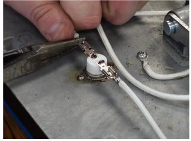
Disconnect the heater wires from the thermostat disc.
