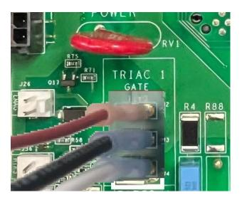
Unplug the ground wire and the 2 wires from the on/off switch from the controller. Depicted image features older power board.
