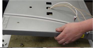
Remove the heater cover and insulation.
