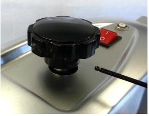
Loosen set screw in shaft of pressure adjustment knob and remove knob using a 1/8th allen wrench.
