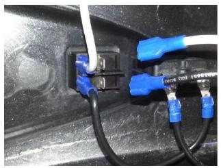
Unplug Black & White wires from Power Switch as shown to disconnect from Controller
