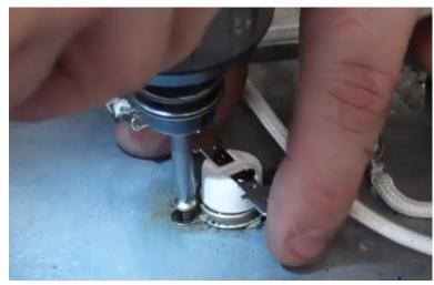
Remove screws to detach the thermostat disc.
