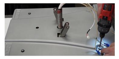
Remove the four phillips screws on heater cover.
