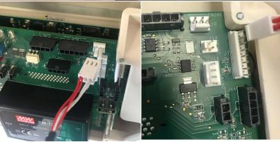
Wire connection for the probe and proxy.
