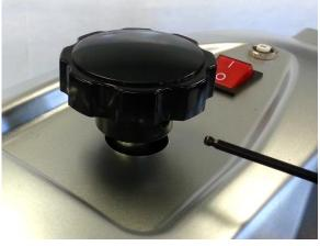
Reattach the pressure knob by tightening the set screw in shaft of pressure adjustment knob using 1/8th Allen Wrench.
