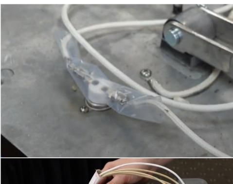
Reattach the thermostat disc, and connect new wire connectors to disc with shrink tube.
