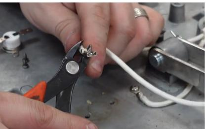
Inspect wires and replace connectors if damaged. Start by cutting off the damaged connector.
