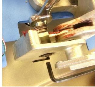
Remove shoulder bolts using 3/16" Allen Wrench and ½" Combination Wrench
